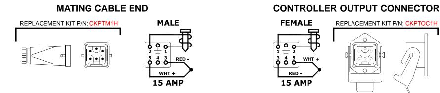
Figure 3 Output Connector Wiring
